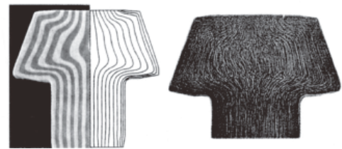
Fig. 2 Comparison of metal flow in differential gear blank, plasticine experiment and FE analysis.
